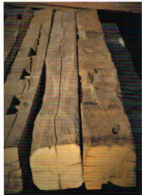
Original belassene Balken in ca. 160 x 160mm
